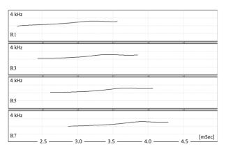
Figure 2. Instantaneous frequencies of dipole Y wave train. Picture shows in line YY component.
