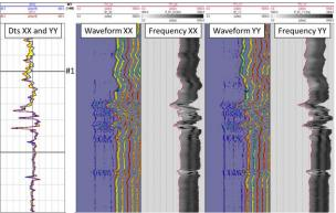
Figure 5. Cross dipole data recorded under anisotropic formation conditions. Track #1 shows flexural wave velocities (DTS XX – blue and DTS YY – brown) obtained with IFS method. Tracks #2 and #3 display raw flexural DXX wave and its instantaneous frequency respectively. Tracks #4 and #5 present dipole YY responses.
