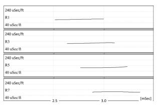
Figure 11. Instantaneous slowness data of monopole wave train recorded at the depth #3 (see Figure 6).
