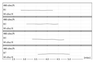
Figure 9. Instantaneous slowness data of dipole XX wave train recorded at the depth #1 (see Figure 5).
