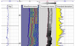
Figure 6. Monopole data recorded under anisotropic formation conditions. Track #1 show compressional wave slowness obtained with IFS method. Tracks #2 and #3 display raw compressional wave and its instantaneous frequency respectively. Track #4 presents standard deviation log computed from slowness distribution.
