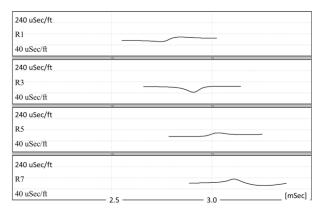
Figure 12. Instantaneous slowness data of monopole wave train recorded at the depth #2 (see Figure 6).
