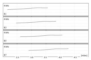
Figure 4. Instantaneous frequencies of dipole X wave train. Picture shows in line XX component.
