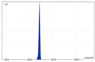
Figure 13. Example of compressional wave slowness distribution derived from high quality data.
