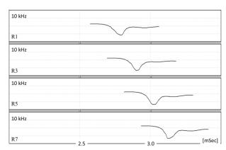
Figure. 7. Instantaneous frequencies of monopole wave train recorded at the depth #2 (see Figure 6).
