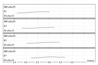
Figure 10. Instantaneous slowness data of dipole YY wave train recorded at the depth #1 (see Figure 5).
